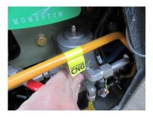
**Step 4**. If steps 1 through 3 do not work, clamp off the hose going into the fuel system and flip the hoes on the IN and OUT connecters.
