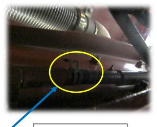
Coolant hose hooks to the metal tubing.
