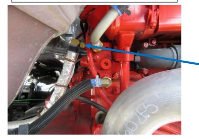
Coolant Supply Port correct tie-in point can be either one of the ports on the Hot/High Side of the engine.
