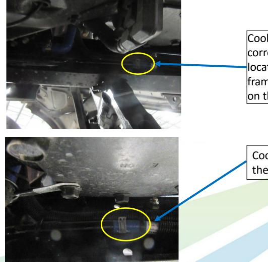
Coolant Return Port correct tie-in point is located between the frame and transmission on the passenger side.
