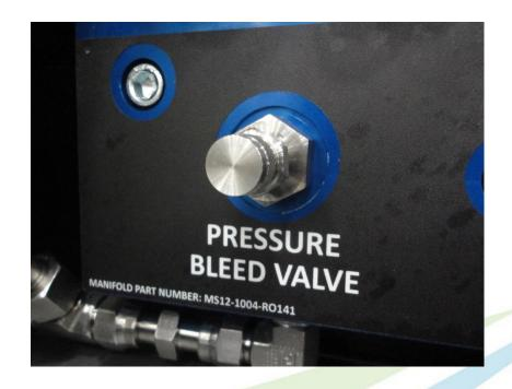
Vent hole bleeds excess liquid or gas from system lines
