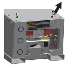
FIGURE 3 - PRD VENT AND VENT CAP
