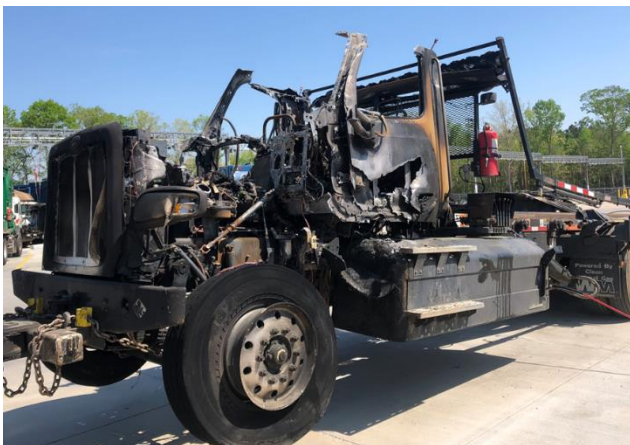
This is an example of a vehicle fire where NO WATER was applied, and the PRDs activated safely.
