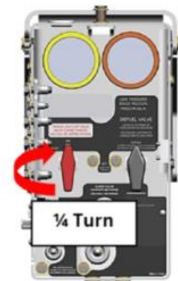
FMM Manual Shutoff Valve
