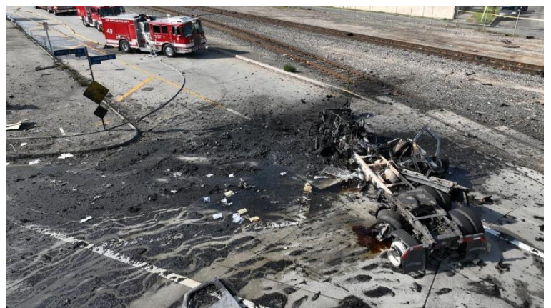
This is an example of a vehicle fire and WATER was applied, and the PRDs DID NOT activate safely.
