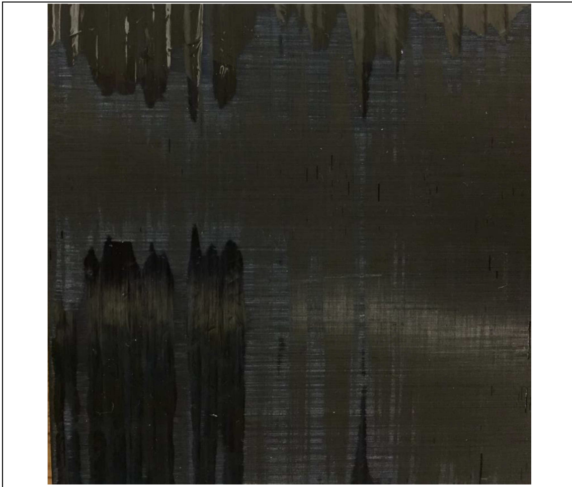
Abrasion marks and scratches
