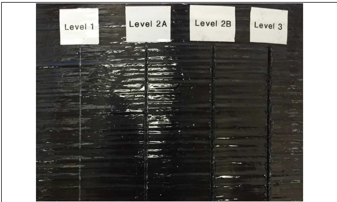
Different levels of cut/scratch damages are shown here. For cuts classified as level 2a and 2b xperion should be contacted
